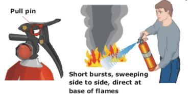
Fire Extinguishers should always be visible, never blocked or used to hang clothing. They should be inspected monthly by checking the pressure gauge, hose, tamper seal, pin and mounting bracket for defects. Dry chemical extinguishers should also be removed from the bracket and turned upside down to loosen the powder during the monthly inspection. Portable fire extinguishers require annual servicing from a professional licensed technician.
