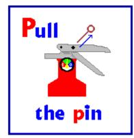
Pull the pin. This will allow you to discharge the extinguisher.
