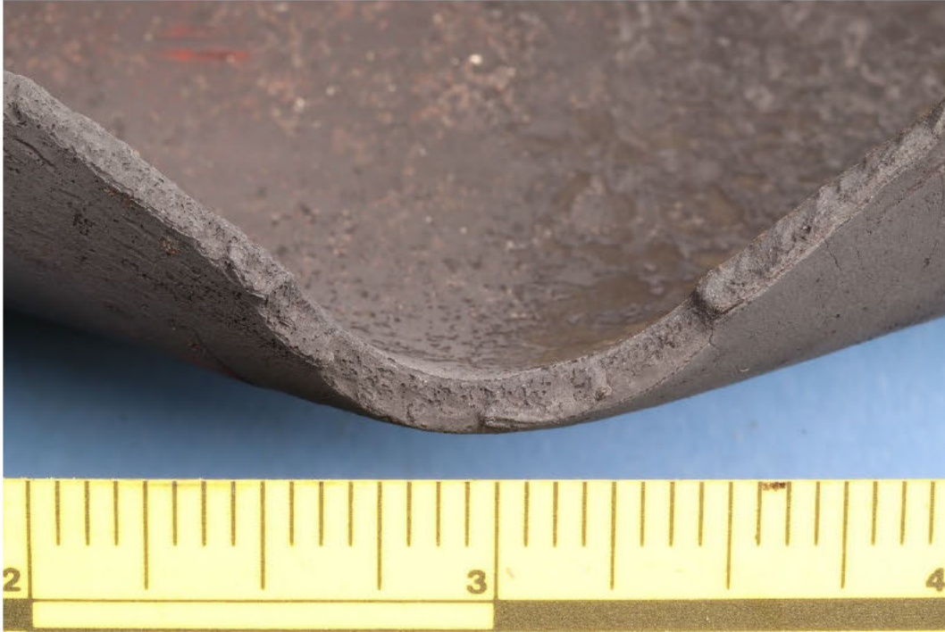
Figure 8. Fracture surface at the center of the longitudinal fracture in pipe B.
