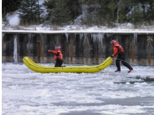
The SKF-ICE is primarily used for ice rescue short-haul cases in enclosed ports, waterways and bays. The construction and inherent design of the SKF-ICE makes this an ideal platform for performing in soft or hard water rescue. The SKF-ICE may be used to transport the ice rescue team to a location to complete the rescue.
