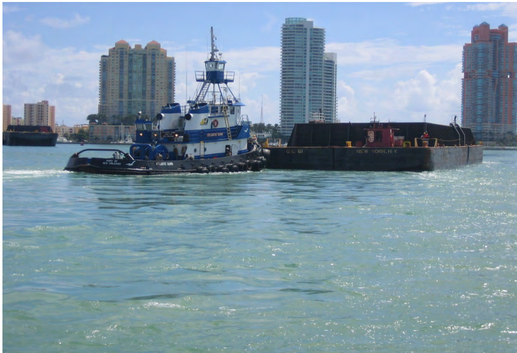
Figure 14 - Split Hull Barge Being Pushed by Tug
