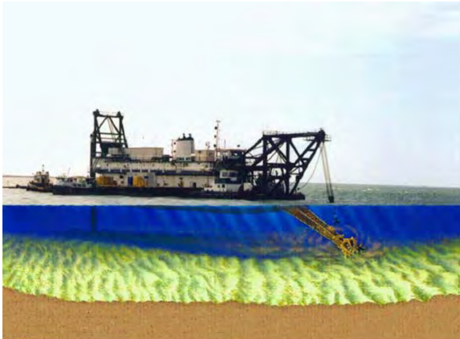
Figure 13 - Cutterhead Dredge Contacting Substrate
