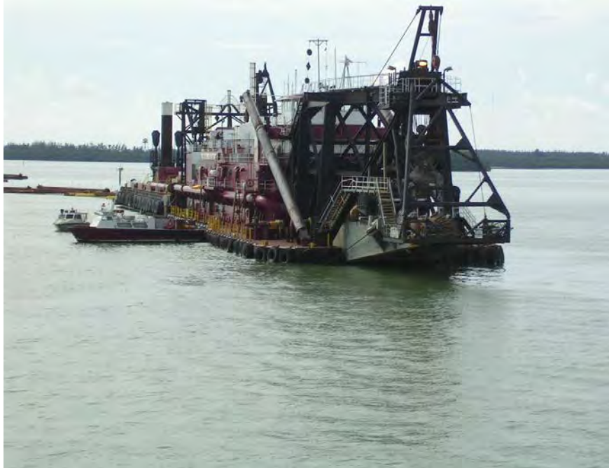
Figure 12 - Hydraulic cutterhead dredge vessel
