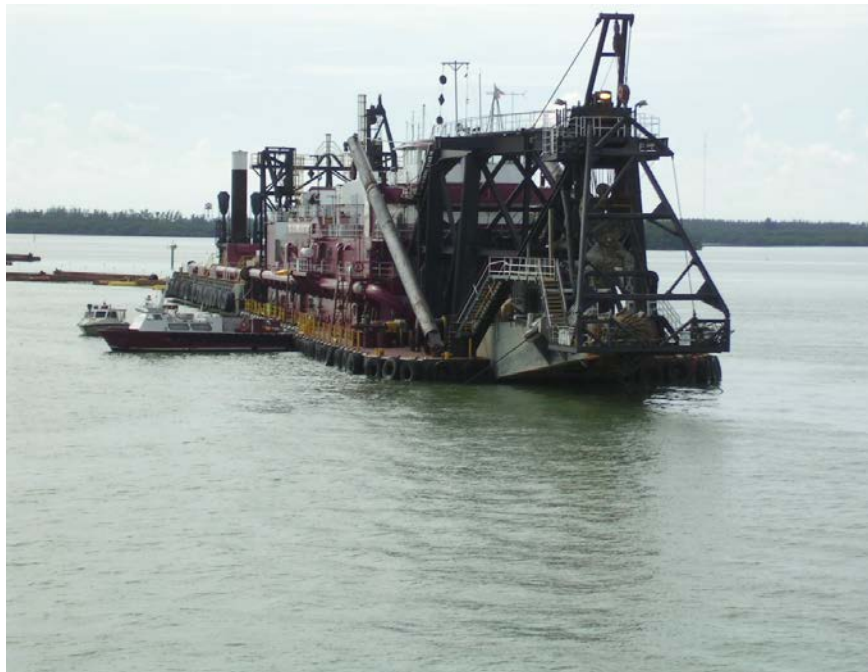
Figure 12 - Hydraulic cutterhead dredge vessel
