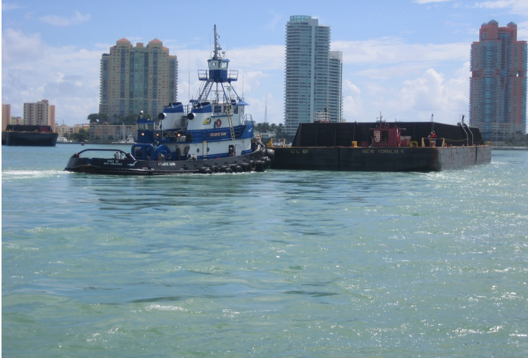
Figure 14 - Split Hull Barge Being Pushed by Tug
