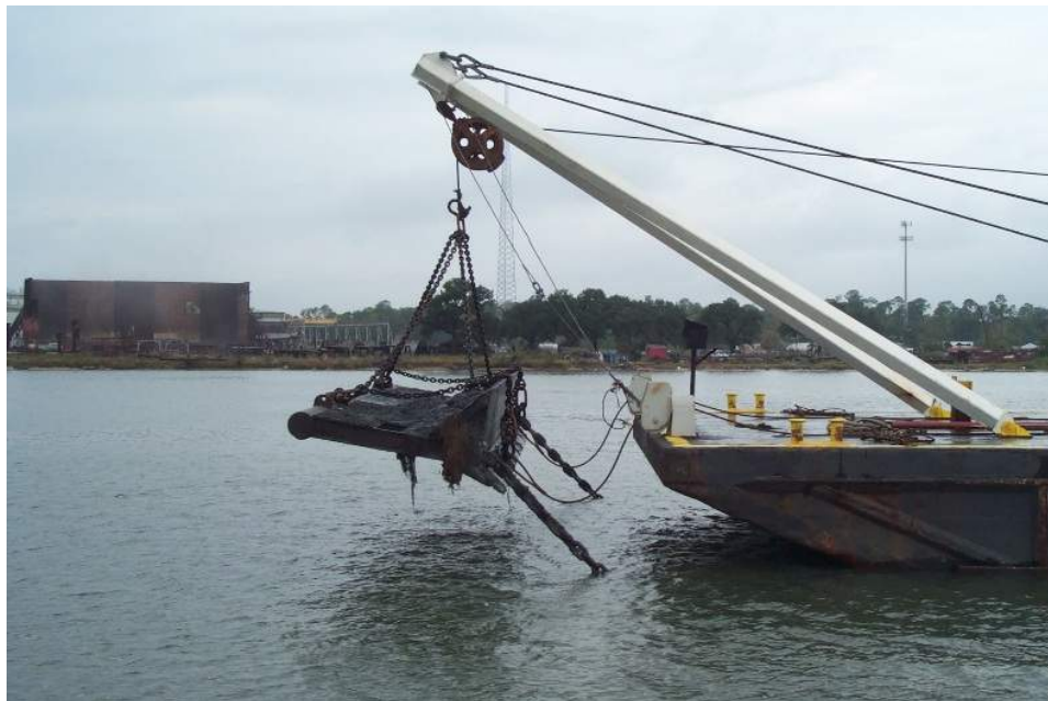
Figure 17 - Davit-mounted Drag Bar
