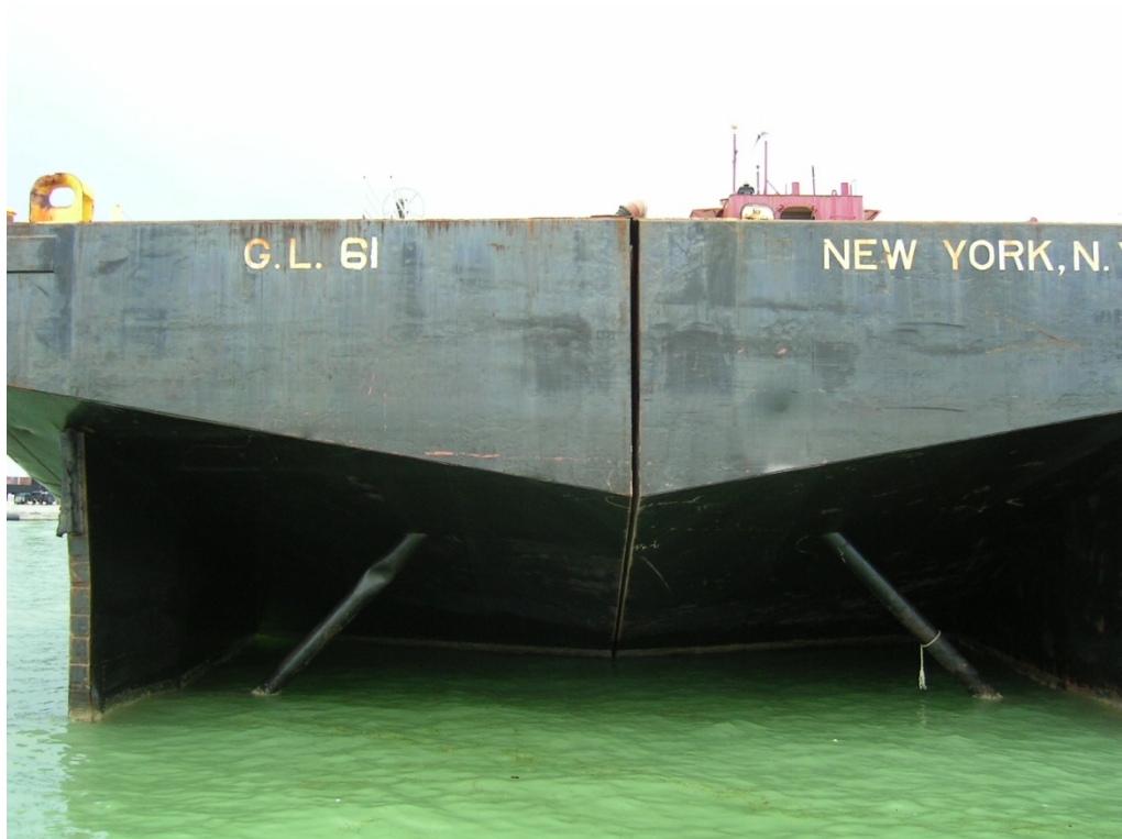
Figure 15 - View of Stern of Split-hull Scow
