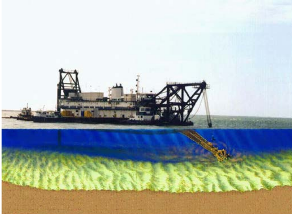
Figure 13 - Cutterhead Dredge Contacting Substrate
